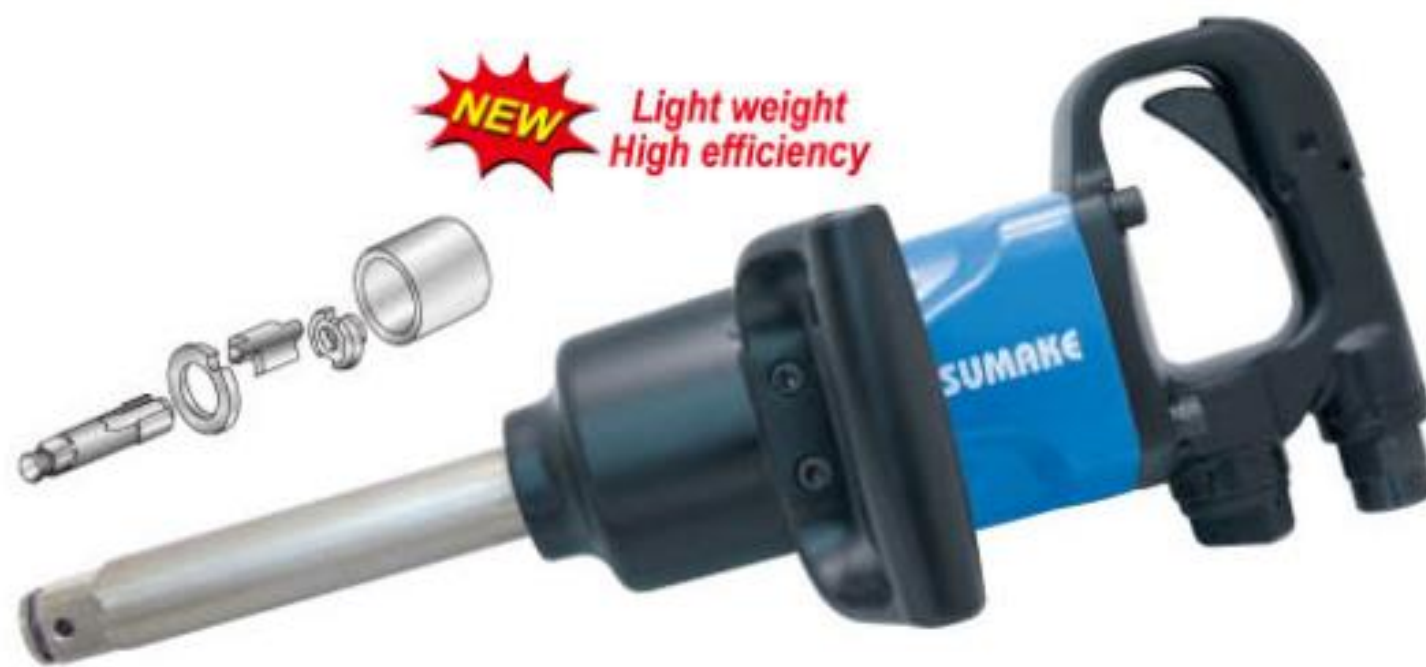
ST-IW1386L-7 1" Dr. w/ 7" Ext. Anvil Max Torque: 2,371Nm (1,750 ft-lb) Pinless Clutch
