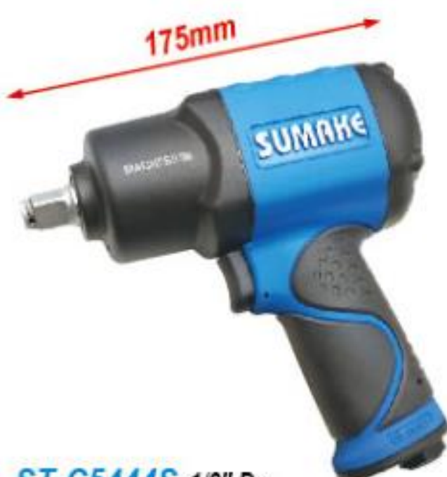
ST-C5444S 1/2" Dr. Max Torque: 1,491 Nm (1,100 ft-lb) Twin Hammer 1.65kgs
